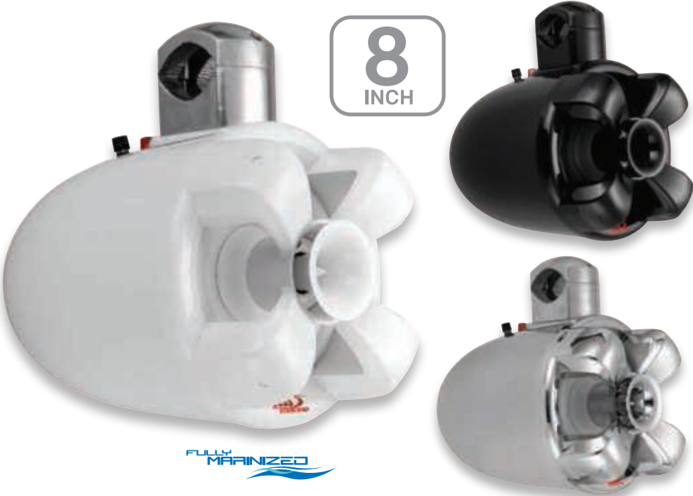
ROCKER 1000 WATTS MAX POWER 3-WAY MARINE WAKETOWER SPEAKER SYSTEM Featuring 8" Midbass and 5-1/4" Midrange Speakers and 1" Bullet Tweeter. 20-9/16" (L) x 11-5/16" (W) x 14" (H) SOLD IN PAIRS
